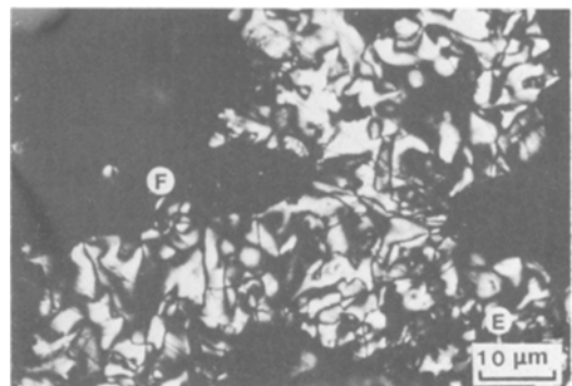
Figure 4 Optical texture of carbon from A240/HA43, 90/10, 200 MPa, showing coarse-grained mosaics (Position E) and botryoidal structures (Position F).
